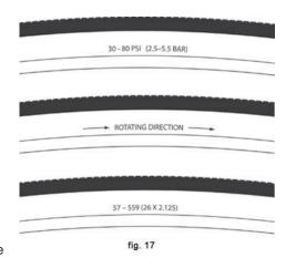
(see fig. 17). The part of this information which is most important to you is Tire Pressure. But some wheel rim manufacturers also specify maximum tire pressure with a label on the rim.
