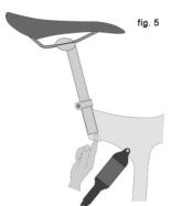
WARNING: When making saddle angle adjustments with a single bolt saddle clamp, always check to make sure that the serrations on the mating surfaces of the clamp are not worn. Worn serrations on the clamp can allow the saddle to move, causing you to lose control and fall.
